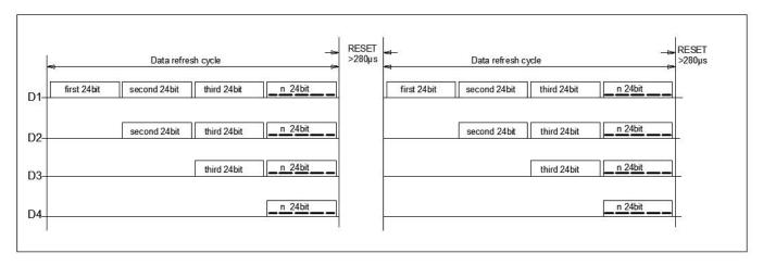
Note: The data of D1 is send by MCU, and D2, D3, D4 through pixel internal reshaping amplification to transmit.
