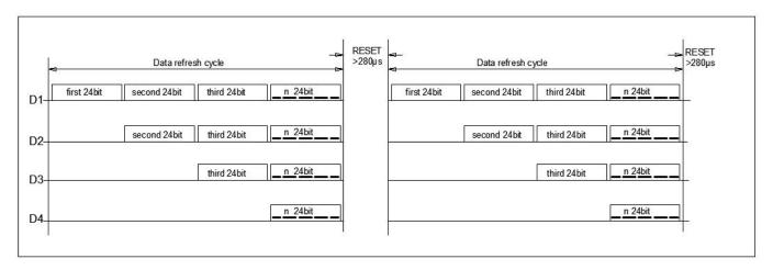
Note: The data of D1 is send by MCU, and D2, D3, D4 through IC internal reshaping amplification to transmit.
