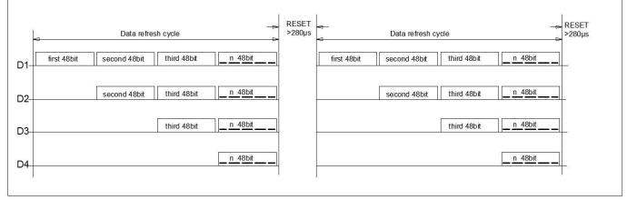
Note: The data of D1 is send by MCU, and D2, D3, D4 through pixel internal reshaping amplification to transmit.
